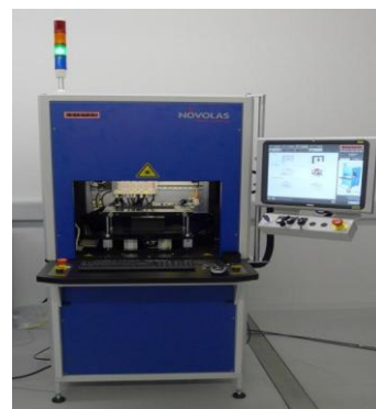
Figure 3: Leister's Dynamic Mask prototype machine with 1070nm fiber laser (YLR-100, IPG) and scanner (MiniScan 20, Raylase)
