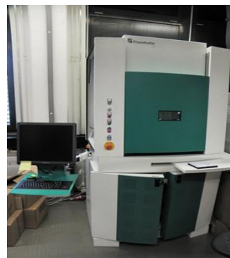
Figure 2: ILT's TWIST prototype machine with 1567nm fiber laser (ELR120, IPG) and scanner (Fiber Rhino 8.5, Arges).
