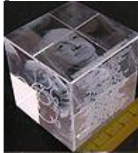
Figure 4: Glass interior engraving with laser radiation
