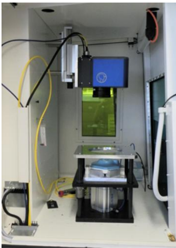
Figure 1: PEEK foil welding setup at ILT with scanner, collimated fiber laser input (yellow) and clamping unit.
