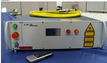
Figure 2: Prototype fiber laser system emitting at \lambda=1567\text{nm}
